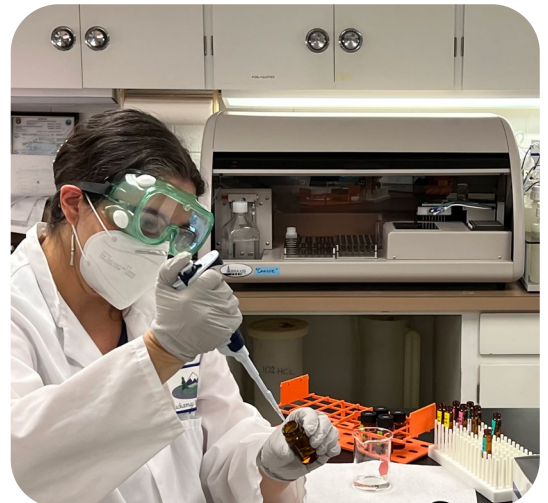
Our source water being tested for cyanotoxins the same day the sample was collected.
