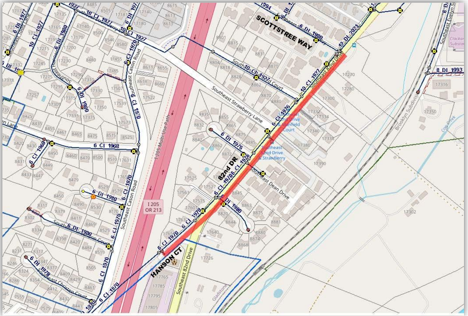
82 nd Drive Waterline – Phase 2 Proposed 12” Waterline
